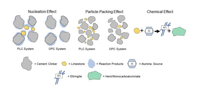
with traditional, OPC-SCM systems.<sup>(31)</sup> This increase in pozzolanic reactions can potentially contribute to reductions in pore connectivity and thus result in improved concrete transport properties (e.g., rapid chloride permeability test (RCPT) or resistivity) of concrete.<sup>(31)</sup>
